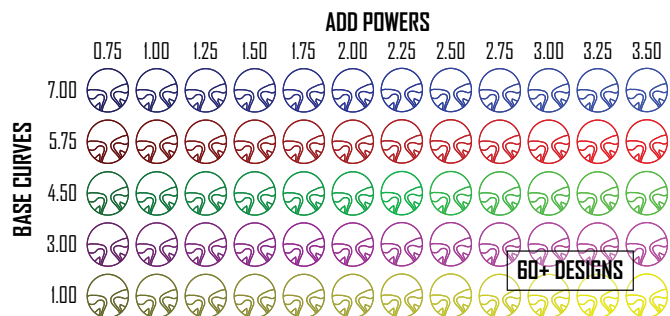
Figure 4. Physiologically Mapped Optics starts with a distinct lens design for each base curve and addition power combination, resulting in 60 or more lens designs.
